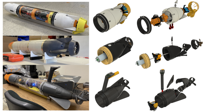
Fig. 3. Photos of the Sea Beaver I, a modified EMATT variant which was named the "Sea Badger", and then the Spurdog AUV, each depicted with the associated aft section which was tested on the vehicle.
