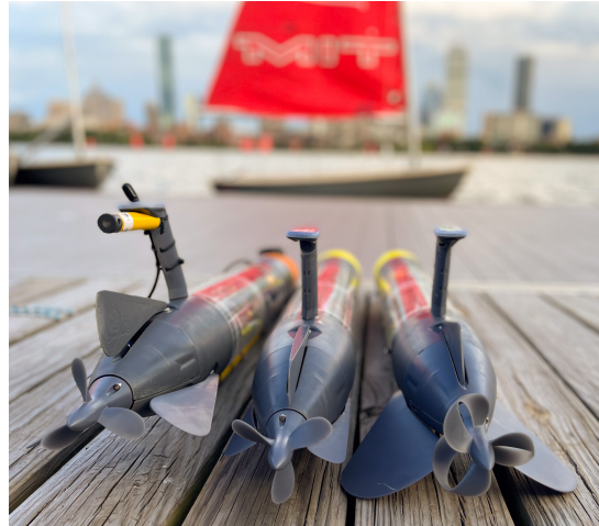
Fig. 1. Photo of three Spurdog AUVs on the dock at the MIT Sailing Pavilion, Cambridge, Massachusetts. The vehicle on the left is pictured with a Sonotronics Pinger mounted to the mast, with a miniature hydrophone. The vehicle in the center, is fitted with the A-Sized fins. The vehicle on the right is fitted with large elevators to support with improved pitch control, and a toroidal propeller, which was evaluated in related ongoing research.
