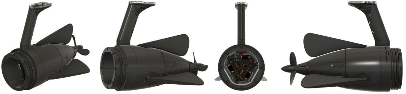
Fig. 2. Four perspective views of the Trident 450 Rev. 1 tailcone, including an optional mast, and the “standard” fins on Spurdog.
