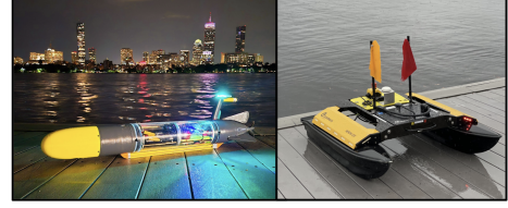
Fig. 4: Platforms used for field experiments: (left) an MIT Spurdog AUV, (right) a Clearpath Heron ASV.
