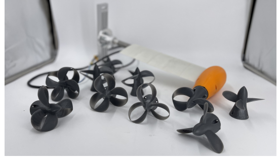
Fig. 1: The propellers tested in this study, and the mounting fixture used in all experiments.
